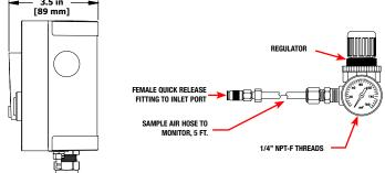
CO-GUARD is supplied with a regulator and 5 foot hose for connection to the monitor. Connection from the facility air supply to the regulator is 1/4 inch NPT female.
