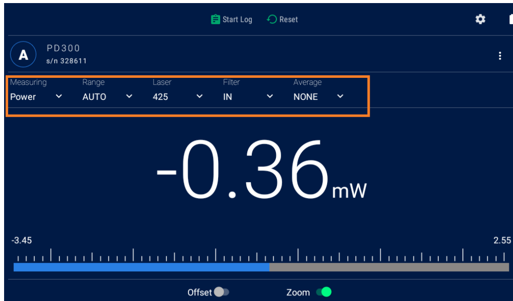
Figure 3-28 Photodiode sensor measurement screen with sensor parameters highlighted
