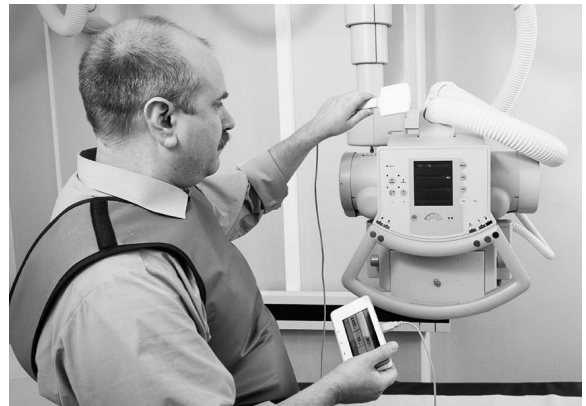
Testing for potential tube leakage.
