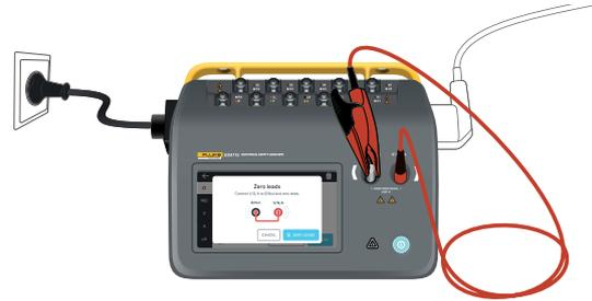
**Figure 9:** Setup for zeroing at protective earth resistance measurements, using one test lead and the null post adapter.
